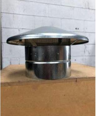
BAL RATING 12.5 - 29 Low level ember attack Fitted with stainless steel mesh. Mesh with max aperture of 2mm Corrosion resistant stainless steel 304 mesh Non combustible All sizes from 100mm - 300mm Zinc & Galv C/bond available on request
